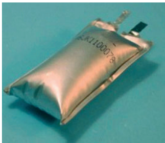
Figure 2: Swelling pouch cell
