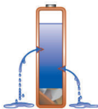
Figure 6: Effects of high self-discharge Self-discharge increases with age, cycling and elevated temperature. Discard a battery if the self-discharge reaches 30 percent in 24 hours.
