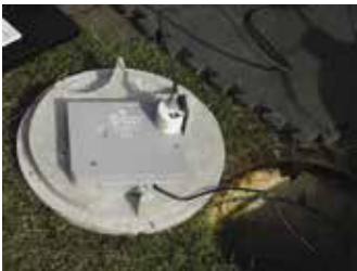
AMR/AMI meter transmitter units (MTU) are often buried underground, exposed to extreme temperatures and difficult to access for replacement. Bobbin-type \text{LiSOCl}_2 cells with passivation minimize the need for future battery replacement, which increases ROI.
